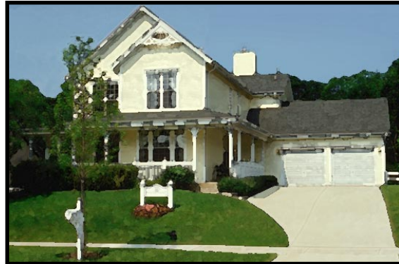
✓ Recessed garage is tied to the main body by the wrap-around porch. The driveway is kept narrow across the front yard.
