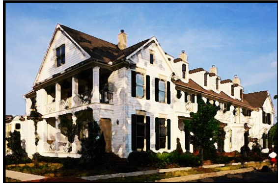
✓ Gable end projections with full length porches provide single-family character to the corner of this building.
