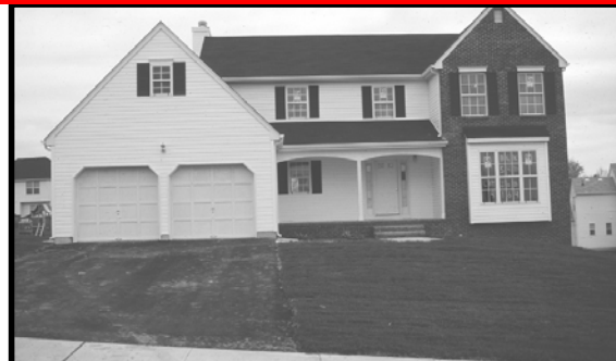
✗ The garage portion of this house extends forward of the main body. The width of the garage gable dominates the front facade, overpowering the porch and brick gable.
