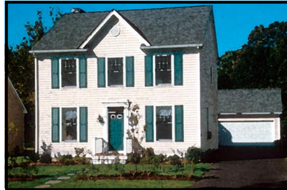
✓ This is a simple, cost-effective building form where details are applied only to the front facade. The attached garage is placed far enough from the street that it does not require screening.
