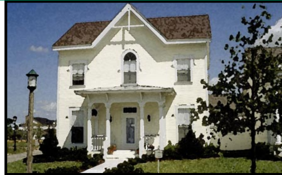
✓ Central focal points such as well detailed porch, Gothic arched window and gable carpentry details highlight the symmetrical facade with center entrance.
