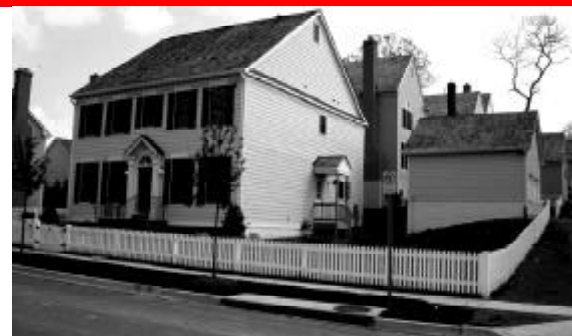
✗ This home has too much blank wall exposed to the side street. Blank wall areas can be treated with taller landscape or trellis in lieu of more expensive architectural elements.
