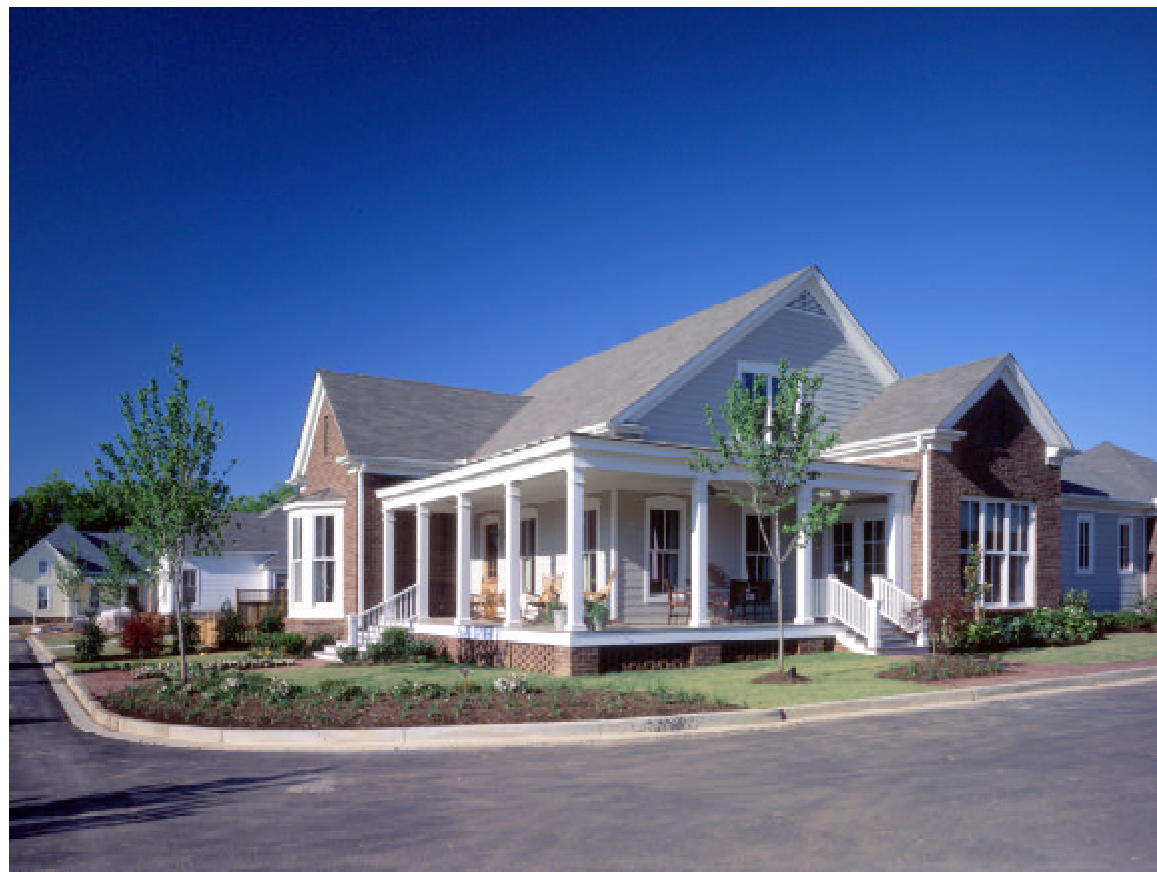
✓ Corner lots have two "front" facades. A lot side that has frontage on a secondary street or communal open space will have front setbacks even if the "front" (formal entrance) of the home faces another street. The Cherry Hill Village Site Plan should be consulted for the setback distances along each street.
