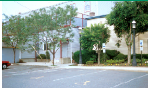
✓ The rear of commercial buildings should have sidewalks for access to street, lighting, and landscaping to soften the parking lot and service areas.
